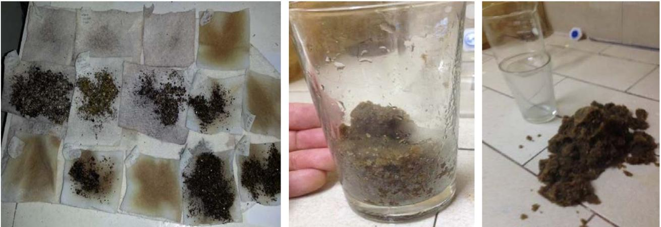
**Samples of Bagacillo and Impurity Filtered out from Juice Streams**
