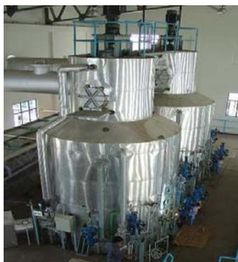
The results of automating a batch pan in this way achieves many benefits including improved crystal quality and reduced recycle of sugar. The elimination of water during boiling is a key advantage, reducing the boiling time and saving steam, all of which assist in making superior sugar in the most efficient manner.
