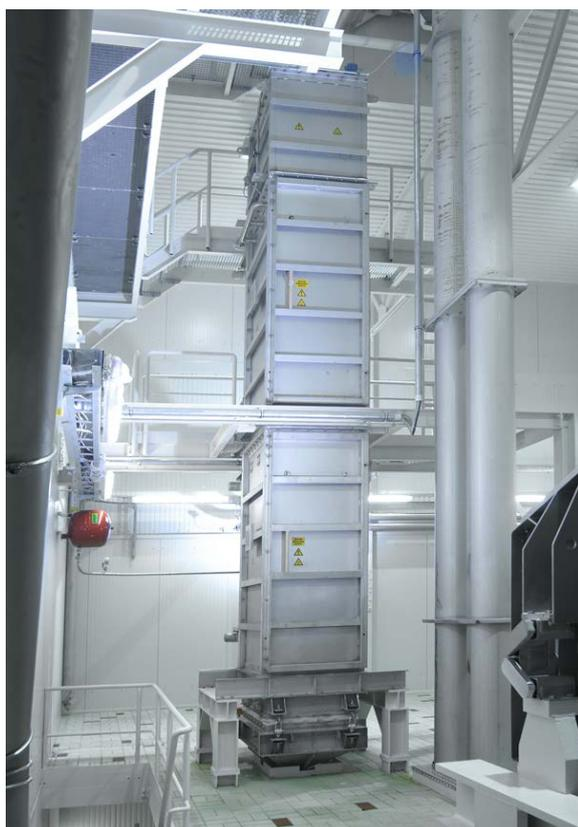
In order to achieve short retention/ rapid conditioning, an advanced combination of specialised sugar drying and indirect contact cooling is combined to provide fast results. In most existing installations, simple modifications to the sugar dryer are all that is required, plus additional conveying equipment and a specialised cooling silo. The cooling silo consists of indirect cooling plates which allow rapid heat transfer for cooling of the sugar while purging with de-humidified air.
